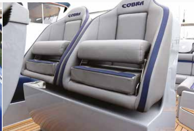
2. The seats have concealed suspension units.
