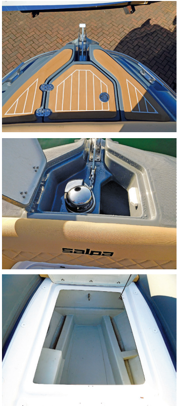
Ergonomically the helm set-up works well. The ‘Med-style’ bow is capped with good-quality synthetic teak. A hidden windlass makes good sense. A huge forward locker and some meaty longitudinal stringers.
