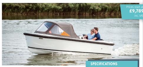
technological upgrades being available, including a Teakline floor and charging facilities. Making good on the Dutch-built boat's hull, designed for stability and an easy cut-through, is a Honda BF20 engine. Advanced features such as a reverse gear and electric start bring userfriendly functionality, which is backed up by a programmed fuel injection system and rubber mountings that make for smoother going.
