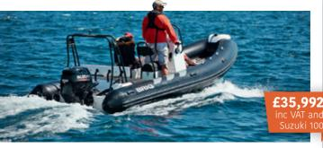
engines and a one-year warranty on fixtures, fittings and accessories. The Navigator 570H comes with BayStar hydraulic steering and the Suzuki DF100. It has teak SeaDek non-slip flooring, a sun deck, and a console and overall cover. The electronics included are a Garmin 115i VHF, EchoMap GPS/plotter and a sounder with transducer. There is also a Fusion RA70 stereo with two speakers.
